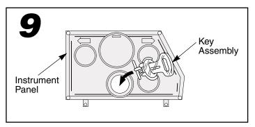
• Snap the key assembly into the hole in the instrument panel.
